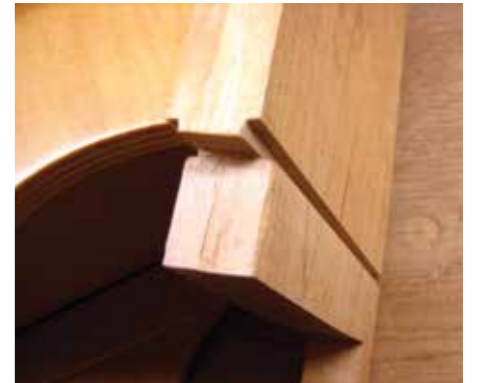
Grooves in the drawer support are used to locate the drawer housing
