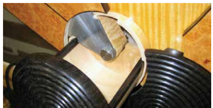
On the Patience cabinet the drawer support also serves as the pivot point for the door
