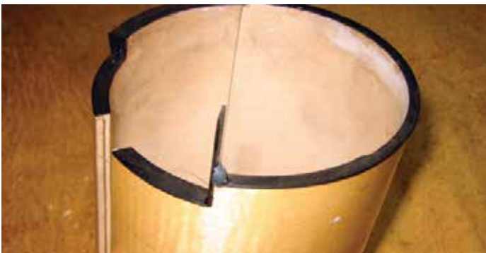
Hot glue is the perfect third hand when conventional clamps don't work
