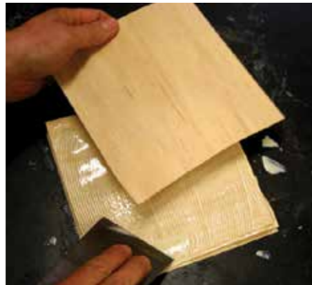
Layer the veneers on top of each other in a sandwich as you work
