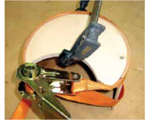
A strap clamp works nicely when gluing the round backs in place
