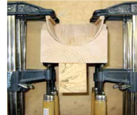
Mount the drawer in a cradle jig to help attach the solid wood lippings
