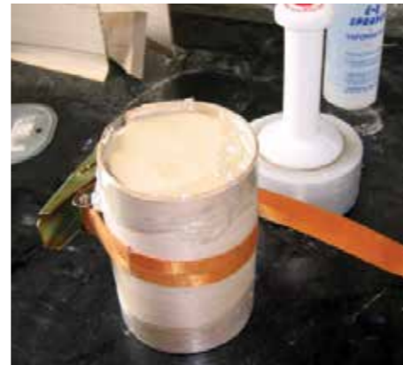
Use whatever means you have at your disposal to hold the veneers onto the former before it goes into the vacuum bag
