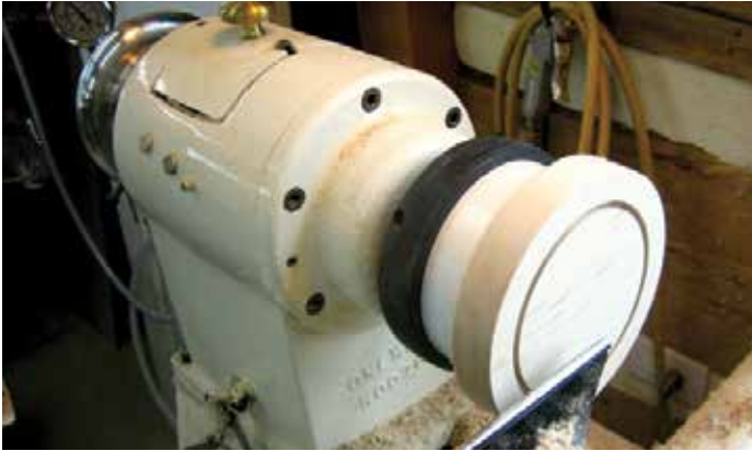
While you've got the drawer front on the lathe, cut the groove for the drawer box
