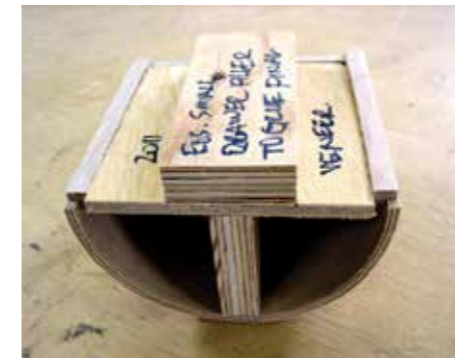
This drawer sizing jig may appear crude but it's an essential part of the build process
