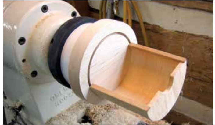
Test fitting the drawer in its groove in the drawer front while the drawer front is still on the lathe
