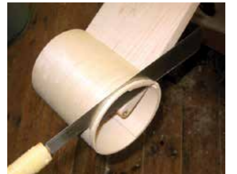
Trimming the housing to length while it hangs on the drawer support
